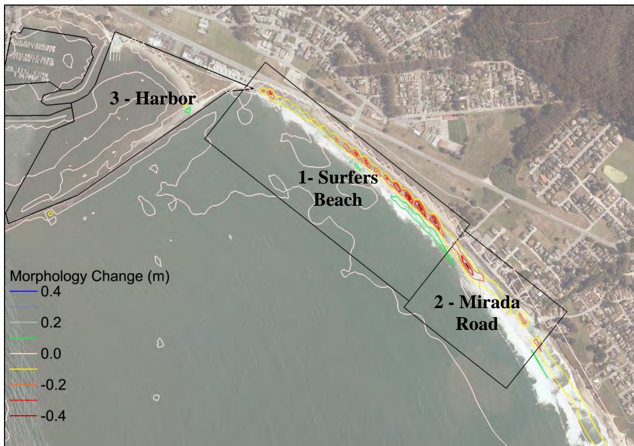
Figure 45. Calculated morphology change in the vicinity of Surfers Beach from June 2009 to November 2009 (6 months) based on a sea level rise of 0.71 ft (0.22 m) in 50 years (USACE Intermediate Rate). The boxes (1 – 3) outline the analysis areas
